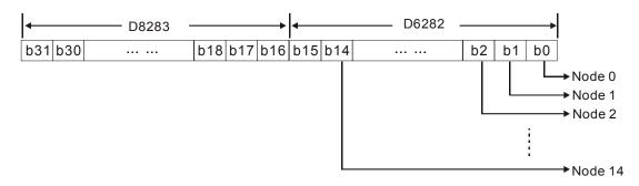
In the bit-strobe mode, the master will not send control data to the slave node. However, when its corresponding bit is set to 0, the slave node will have to respond with I/O data to the master. When its corresponding bit is set to 1, the slave node will not have to respond with I/O data to the master.
