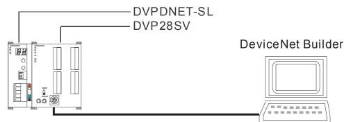
Open DeviceNet Builder software and select "Setup" => "Communication Setting" => "System Channel". And then the following dialog box appears.
