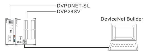
Open DeviceNet Builder software, and select "Setup" => "Communication Setting" => "System Channel", and the "Serial Port Setting" dialog box will appear as below.
