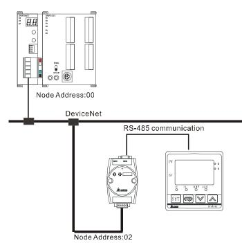
Note: IFD9502, a Delta DeviceNet slave module can connect the temperature controller to DeviceNet network.
