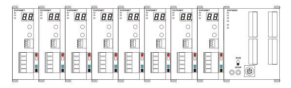
The index of DVPDNET-SL is its unit number. The first DVPDNET-SL on the left hand side of DVP-SV is No. 1, the following DVPDNET-SL modules are No. 2, No. 3, No. 4 and so on.
