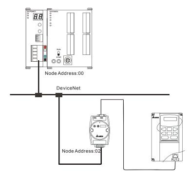
Note: IFD9502, a Delta DeviceNet slave module can connect VFD AC motor drive to DeviceNet network.
