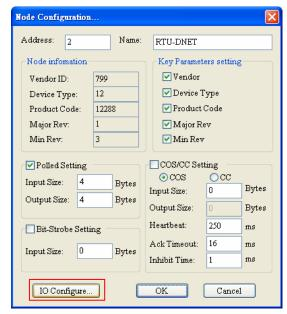
5> Double click on RTU-DNET (node 02), and the "Node Configuration..." dialog box will appear.
