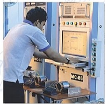
Surge Impedance Test
