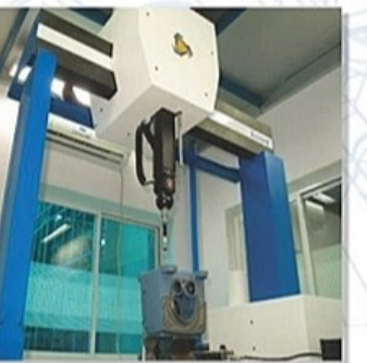
CMM for mechanical inspection
