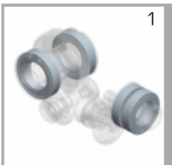
1 ZZ per-lubricated bearings on input and output shaft
